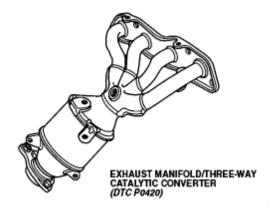
One TWC is near the cylinder head, and it's part of the <u>exhaust manifold</u>. If it fails, it causes DTC P0420 (catalyst system efficiency below threshold) to set
